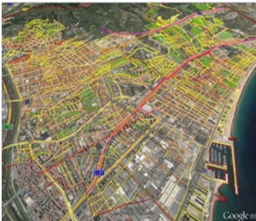
MES of the agglomeration of Barcelonès II. Daily noise index. Google Earth view
